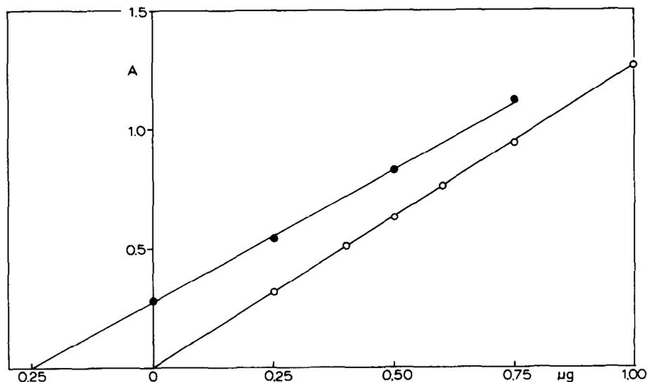
Fig. 3. Calibration graph (area count vs. analyte amount) for phylloquinone (○) and graph obtained by means of the standard addition method (●) applied to oil sample 1. The area count values, multiplied by  $10^5$ , correspond to the output of the integrator used.
