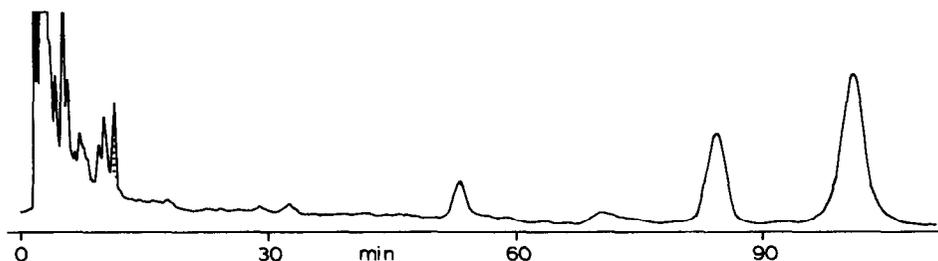
Fig. 1. Chromatogram of a sample (1) from soy bean oil (extract after enzymatic digestion, without LSC). The marked peak corresponds to the partially resolved vitamin K<sub>1</sub>. Isocratic mobile phase: methanol-acetonitrile-water (88:10:2), flow-rate 1.5 ml/min. Detection wavelength: 270 nm. Amount injected: 25  $\mu$ l.
