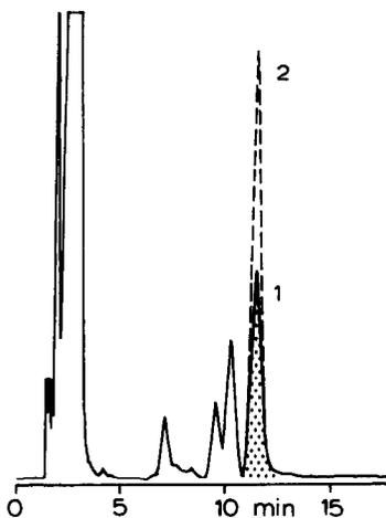
Fig. 2. Chromatogram of a sample (1) from soy bean oil (extract after enzymatic digestion and purification by LSC on alumina). Peaks: 1 = vitamin  $K_1$  endogenous to the oil; 2 = endogenous vitamin  $K_1$  plus vitamin  $K_1$  added ( $50 \mu\text{g}$  to the sample, *i.e.*,  $0.25 \mu\text{g}$  in  $25 \mu\text{l}$ ) for determining recovery. Chromatographic conditions as in Fig. 1.
